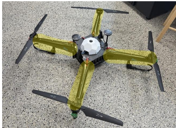
Figure 5 Drone "Arms" highlighted in yellow
