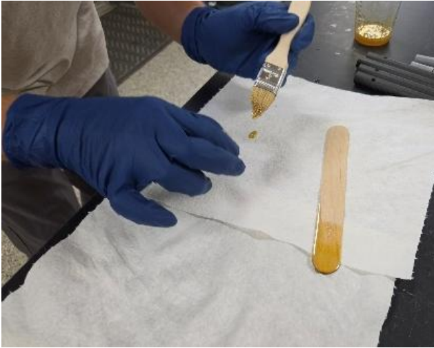
Figure 1 Applying cyanoacrylate glue to a heat-set insert
